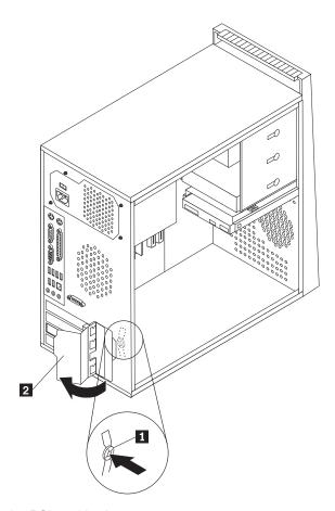
Figure 8. Opening the PCI card latch
